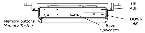
Press and hold these buttons to adjust height into a desired position. If you release the button the height adjustment will stop.
