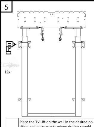
Place the TV Lift on the wall in the desired position and make marks where drilling should be carried out.
