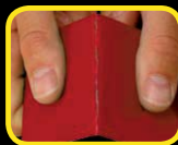
Brand X Cracks and flakes when bent
