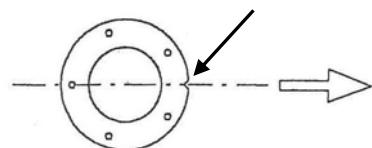
Notch for alignment of free-arm sunshades. Align the notch towards the middle of the seating area.
