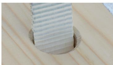
Loch bohren (Ø 35–40 mm)
